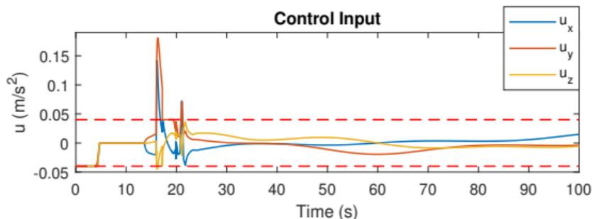
Figure: The control input using  $H_o(x)$  from prior work, which necessitates using control inputs outside the prescribed bounds (dashed red lines) for the QP to have a solution
